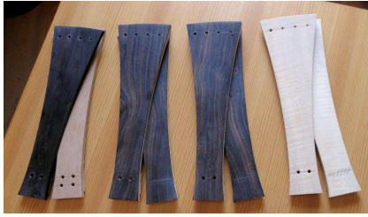
Figure 13: View from upper surface of the eight tailpieces made on the same outline. , two are in plain maple, two covered by thin 1.8 mm of A. Blackwood adjusted shell, two with thick 1.8 mm of A. Blackwood adjusted shell. One is in plain blackwood, and N°1 is in hardwood (Massaranduba) weighing 70g.
