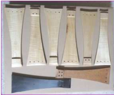
Figure 14bis: View from underneath surface of the eight tailpieces made on the same outline.
