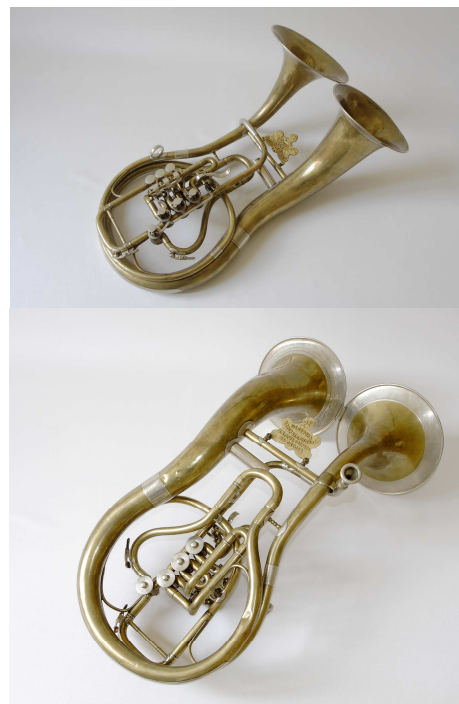
Figure 2 a,b: the alto Eb schediphone used for measurements. The distribution valve is the fourth on the bottom picture and its lever could be seen above the valves on the upper picture.
