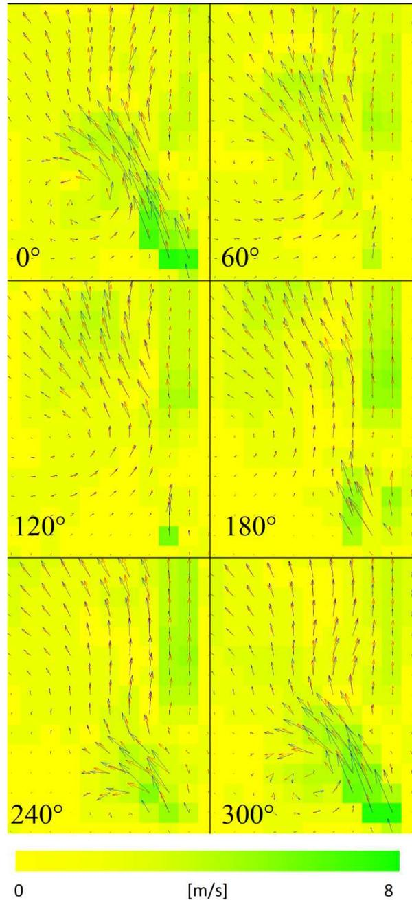
Figure 10: velocity maps in front of the mouth observed from side view in specific phases of generated sound, underlying color corresponds to the local velocity difference between baroque and romantic nicks
