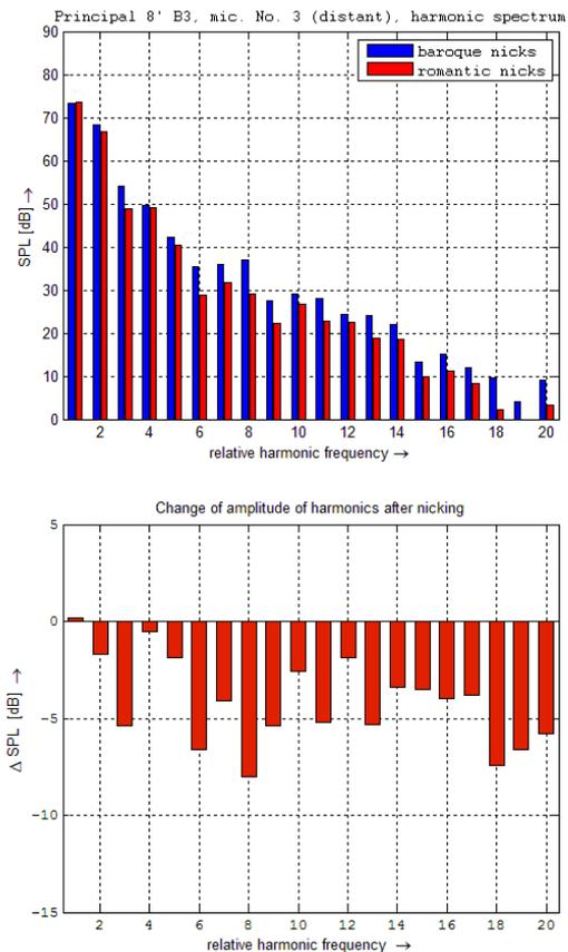
Figure 7: harmonic spectrum of sound of the flue pipe with baroque nicks and with romantic nicks (up), change of the amplitude of harmonics after nicking (down).
