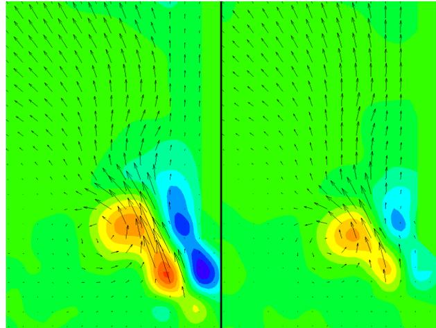
Figure 12: vorticity maps in front of the mouth observed from side view. Baroque mouth (left), romantic mouth (right). Blue, resp. red colors represent negative, resp. positive values.
