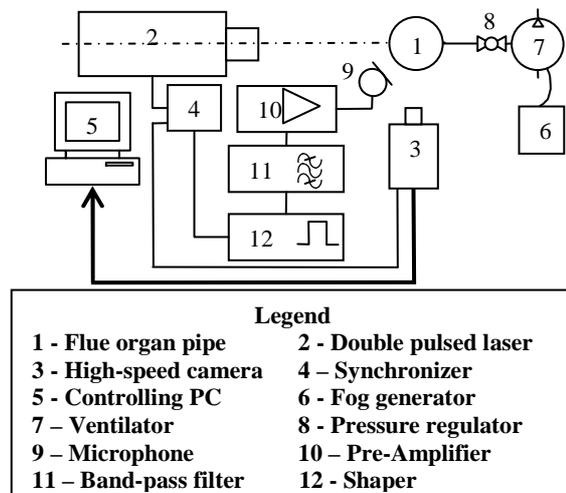
Figure 5: optical measurement setup
