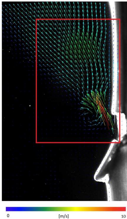
Figure 8: The area of interest in front of the mouth from the side view with averaged velocity vector map in 0°.
