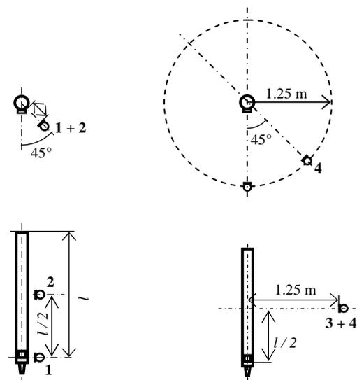
Figure 2: microphone arrangement during pipe sound recording
