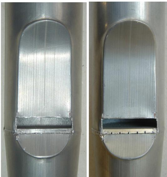
Figure 1: detailed view of pipe mouth; languid with small baroque nicks (left), and with large romantic nicks (right)
