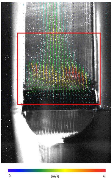
Figure 9: The area of interest in front of the mouth from the front view with averaged velocity vector map in 0°.
