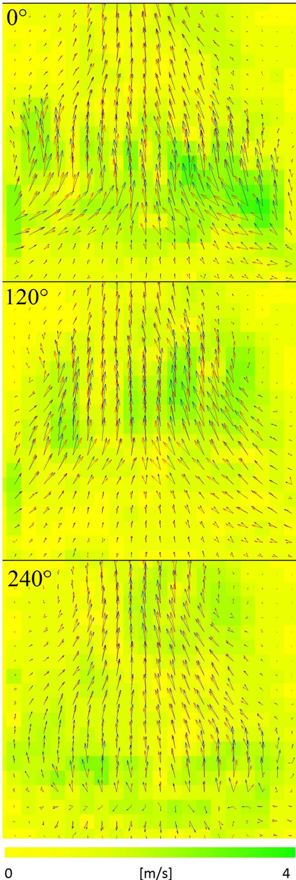
Figure 11: Velocity maps in front of the mouth observed from front view in specific phase states of generated sound.
