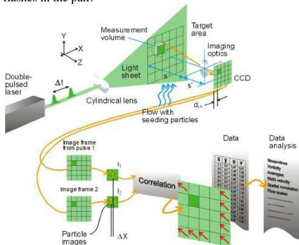
Figure 3: principle of Particle Image Velocimetry [2].
