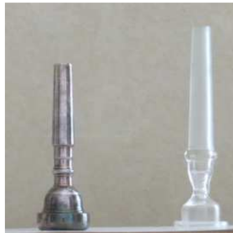
Fig. 1 – Common trumpet mouthpiece and glass model used for measurement.
