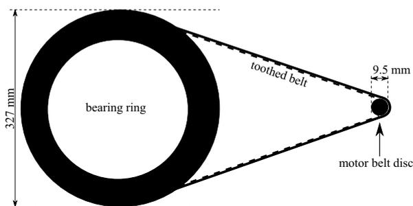
Figure 4: Example of a gear belt drive with a reduction of about 1:35.
