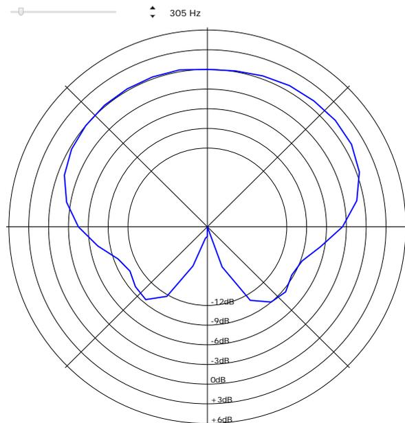
Figure 9: Directivity pattern of a tuba in B at 305 Hz
