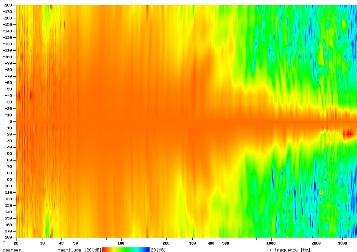
Figure 10: Directivity sonogram of a Tuba in B, Ceiling: 120 dB, Floor: 20 dB, f-min: 20 Hz, f-max: 3962 Hz and 0 degree measurement positioned in the horizontal centre.
