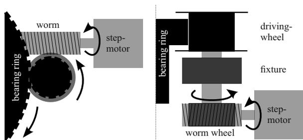
Figure 5: Principle of the designed gearing mechanism. Left: ground plan, right: sheer plan.
