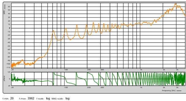
Figure 8: Single transfer response of a tuba in B
