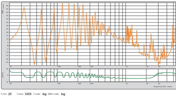
Figure 7: Input impedance of a tuba in B
