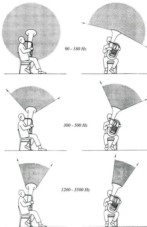
Figure 2: Main radiation area (0 to -3 dB) of a Tuba by Meyer [3].
