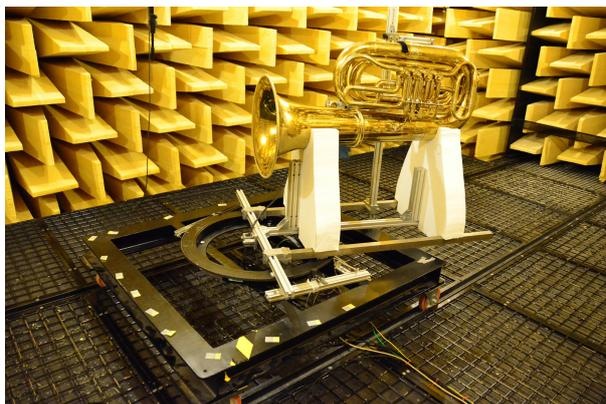
Figure 3: Turntable system with a stable construction for fixing a Tuba.
