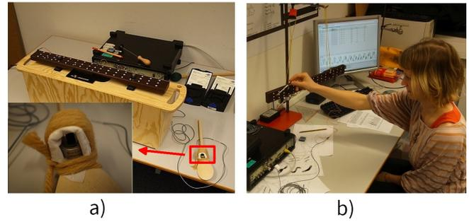
Figure 2: Comparison measurements with an accelerometer
