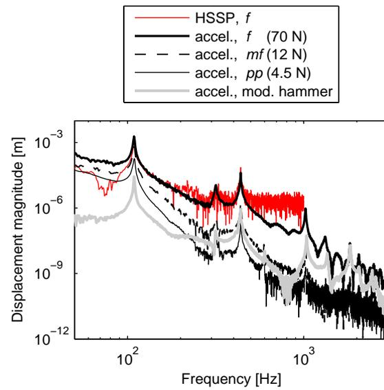
Figure 4: Displacement magnitudes of the Chime Bar directly measured with HSSP and integrated from accelerometer measurements. The bar is struck with a normal mallet (HSSP), a modified mallet equipped with force sensor, and a modal hammer. Values in brackets are the peak forces measured with modified mallet.
