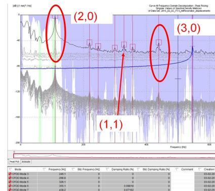
Figure 5: Screenshot of the Modal Analysis (OMA) on high-speed stereophotogrammetry data of a struck Chime Bar using the Brüel&Kjær's software PULSE Labshop.
