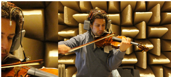
Figure 3: Left: Microphone attached to a violin in the laboratory study. Right: Violinist playing in a simulated concert hall while wearing extra-aural headphones.
