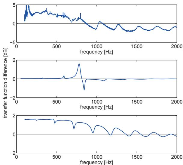
Figure 3: (Top) Difference in the acoustic transfer functions shown in Fig. 2b. The crossover frequency occurs at approximately 860 Hz. (Middle) Calculated difference in the ATF using the model described in Ref. [1]. (Bottom) Calculated difference in the ATF including the gap between the bell and baffle. Details are given in the text.
