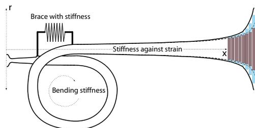
Figure 1: Diagram of a brass wind instrument and how axial vibrations can cause changes in the bore diameter. (After Ref. 1)
