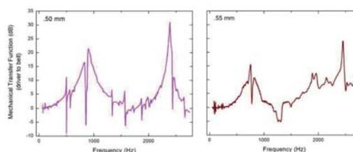
Figure 4: Axial MTF from mouthpiece to bell of the two trumpet bells. The transfer function for the 0.50 mm thick bell was measured using accelerometers and the measurements of the 0.55 mm thick bell were made using a laser Doppler vibrometer.
