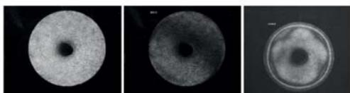
Figure 5: Decorrelated electronic speckle pattern interferograms of the bell with (a) no excitation, (b) oscillating at the first axial resonance frequency (883 Hz) and (c) oscillating at the second axial resonance frequency (2451 Hz).
