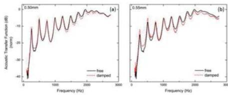
Figure 2: Acoustic transfer function of two straight bells with mouthpieces for the case of the bell freely vibrating (solid) and with the bell heavily damped with bags of sand (dashed).
