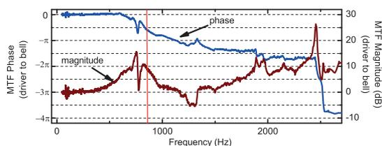
Figure 6: The phase and amplitude of the MTF of the 0.55 mm thick bell. The vertical line indicates the crossover frequency of the ATF seen in Fig. 3.
