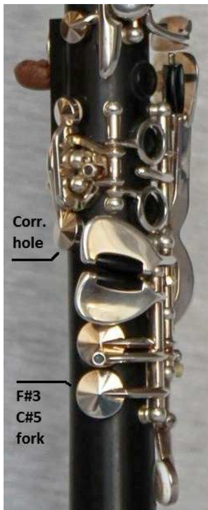
Fig. 10, Detail of the right hand side, showing the two additional holes
