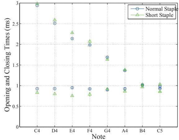
Figure 4: Opening and closing times of an oboe played with a standard staple and reed assembly and with a short staple and bigger reed.
