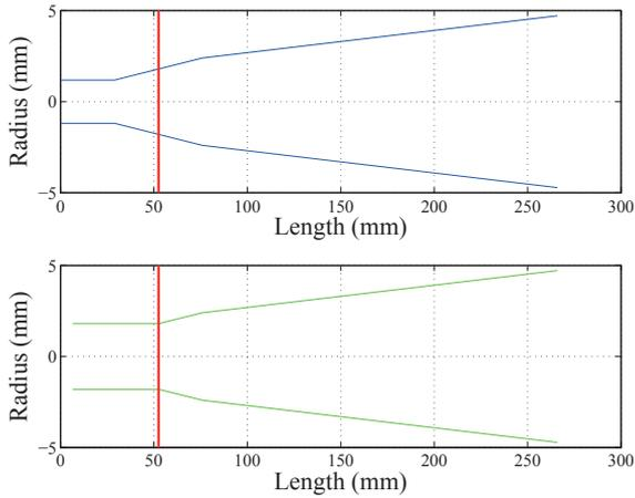
Figure 2: Configuration of staple plus main cone corresponding to note B<sub>4</sub> of the Oboe (top) and Modified Oboe (bottom). The red vertical line shows the point at which the normal staple was cut short.
