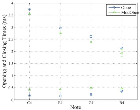
Figure 3: Opening and closing times of a simulated Oboe (short truncation) and a Modified Oboe (long truncation).
