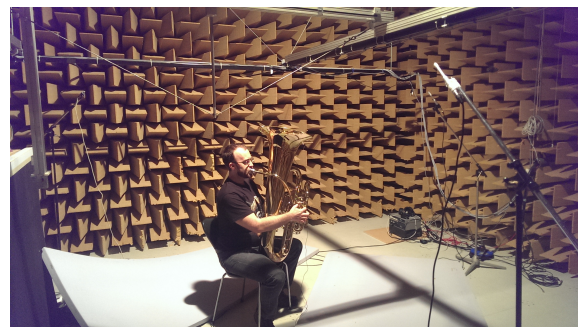
Figure 5: Recording setup in anechoic room using 3 microphones.
